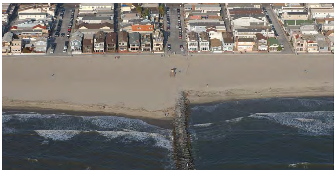
Groin, Newport Beach. Copyright (C) 2004 Kenneth & Gabrielle Adelman, California Coastal Records Project
