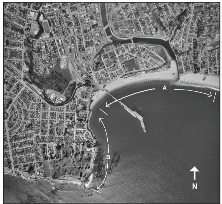
Figure 5.2. The coastline of northern Monterey Bay at Santa Cruz illustrating how the orientation of the coastline determines whether or not a beach forms. Where the shoreline is oriented essentially east-west and littoral barrier exist (A), wide stable beaches have formed. Where the coastline is oriented essentially north-south and there is no barrier, beaches rarely form (B). North is up in the photograph.
