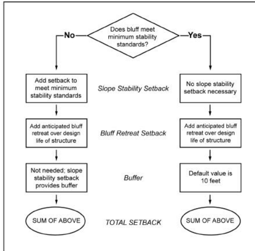
Figure 6. Flowchart for establishing bluff edge setback for development, taking into account stability of the bluff, long-term bluff retreat, and uncertainty in the analysis.
